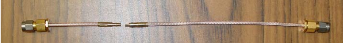
Figure 1 Insertion Loss and VSWR test unit
