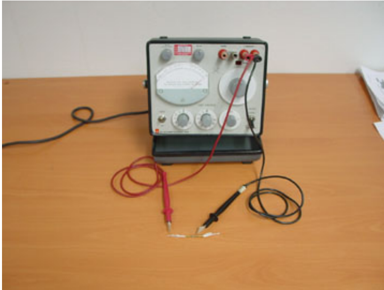
Figure 4 Insulation Resistance Test Set Up.
