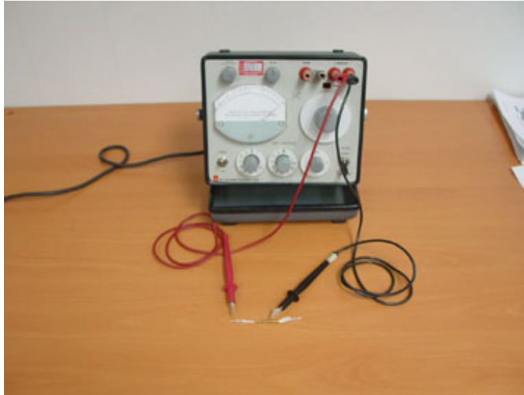
Figure 4 Insulation Resistance Test Set Up.
